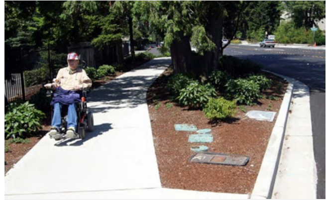
Figure 5-11. Buffered Sidewalk Example
